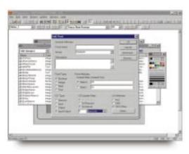
CX-Supervisor assist the user in every detail of the design process. Points are added by using the Add Point dialogue box. This dialogue box contains all selections that need to be made.
